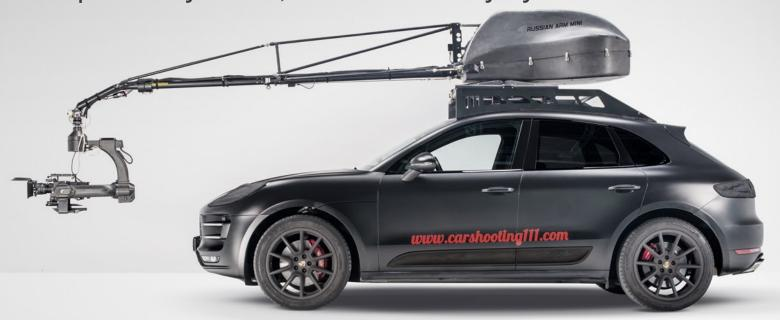
The Russian Arm Mini is lightweight and compact but powerful enough to go high speed and work in most challenging conditions.
