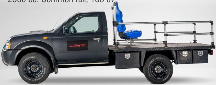
Compact Camera car ideal for Car shoots where a small camera is required. Fully equipped for easy grip with 48 mm aluminum tubular structure, platforms and various adapters.
