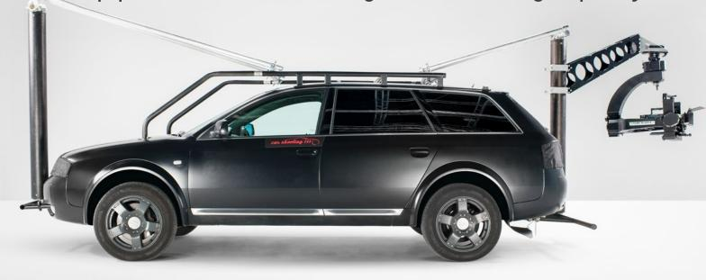
It is ideal to work with any type of remote head on both front and back through the outfitted 48 mm speed-rail pipe with quick-release fittings.
