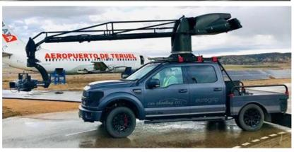
The U-Crane 6 is a stabilized camera crane system that can be mounted on the roof of a camera car or a specialized vehicle which ensures that 360° pan movements can be made while you can also lift up and down.
