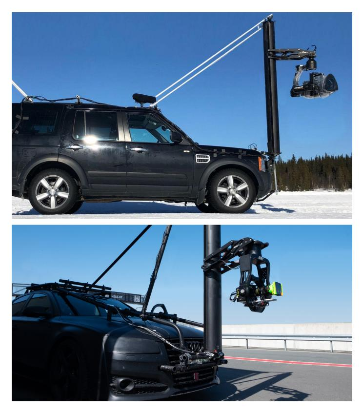
The Tower 24 is a vertical Lifter for Remoteheads and can be mounted on camera cars and or even used stationary. The Tower can be used in conjunction with our Flighthead Mini V4 and V5 and controlled by the camera operator via joystick or foot pedal. The Tower is available to rent separately with a driver and technician as well as a full package which includes the Porsche Cayenne and equipment as listed below.
