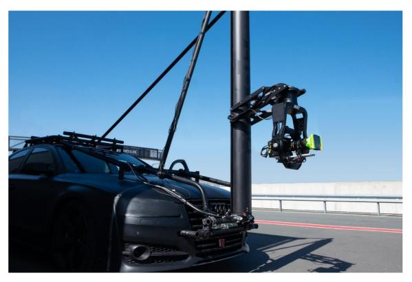
**Total weight of Tower & Shockabsorver**: 34 Kg (75lbs) **Maximum payload of the Absorver Arm:** 30 Kg (66lbs)
