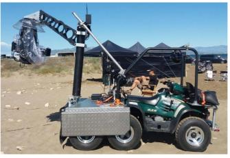
Vehicle designed to capture moving scenes in locations inaccessible or off road (tracks, mountain, beach, etc ...). Both the front and back, is prepared with platform high strength aluminum, to work with 48.3 mm tubular structure. Also has wheel arch protectors. We have a caterpillar to work in extreme snow and mud. Very handy for various uses: from working with steadicam operators, as well as to work freehand with various remote heads.
