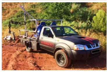
This vehicle is definitely ideal for Car shoots where a small camera is required. Full equipped for easy grip, tubular structure with 48 mm aluminum, platforms and various adapters.
