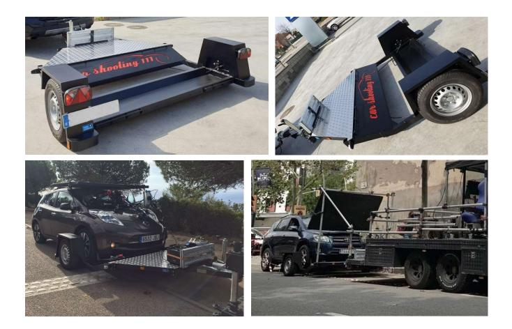
Designed to tow cars as well as motorcycles or bicycles at a minimum distance from the ground, it allows any rig in its 48mm pipe.
